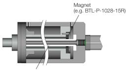
Supporting rod made of non-magnetizable material
