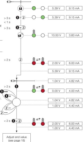
1) Briefly press button: Current value is increased or decreased by approx. 1 mV or 1  $\mu$ A. If a button is held down longer than 1 s, the step interval is increased.
