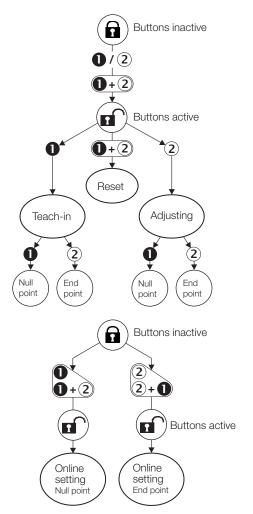
Fig. 6-6: Selecting the calibration procedure
