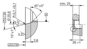
Fig. 4-4: Mounting hole 3/4" 16UNF per SAE J475 O-ring 15.3x2.4
