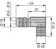
Fig. 12-3: Connector type BKS-S33M-00
