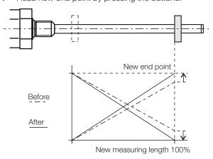
Fig. 6-3: Reading new end point (changing the output gradient)
