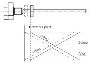
Fig. 6-2: Reading new null point (offset shift)
