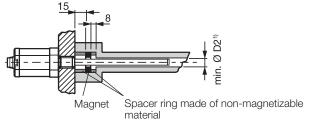
$^{1)}$  Min. Ø D2 = Minimum diameter of the bore (see Tab. 4-1)
