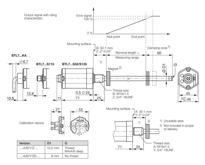
Fig. 3-1: BTL7...A/B/Y/Z(8)... transducer, construction and function
