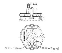
Fig. 6-1: Calibration device in place
