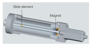
Fig. 4-5: Example 1, transducer installed with sliding element
