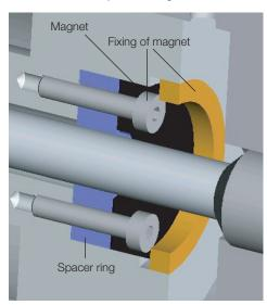
Fig. 4-7: Fixing the magnet
