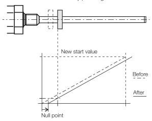
Fig. 6-4: Adjusting new start position (offset shift)
