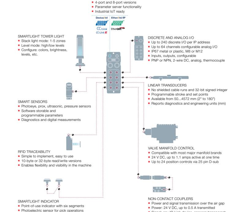
Expansion mode allows two indicators on one port
