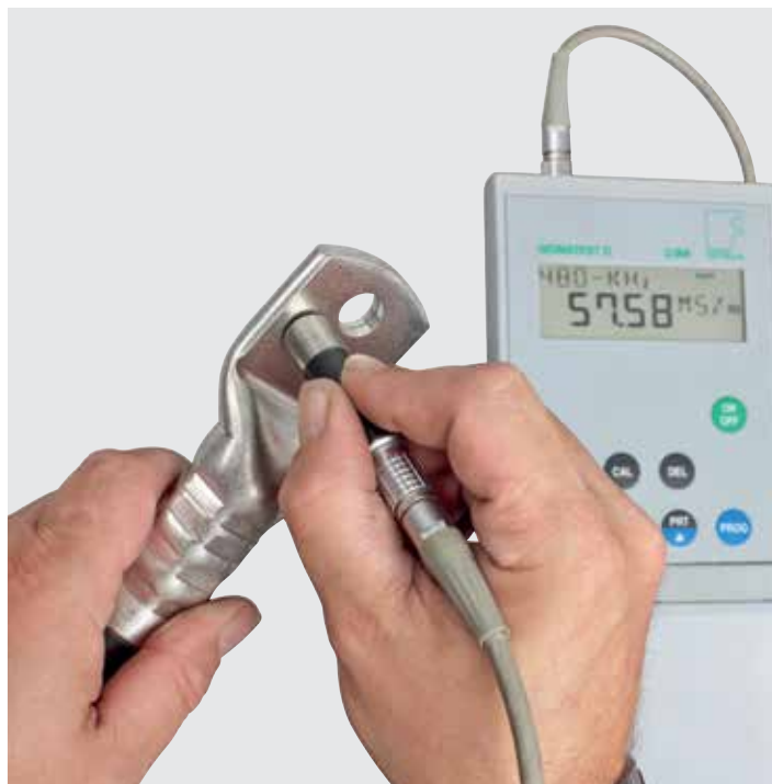
Testing of the conductivity
