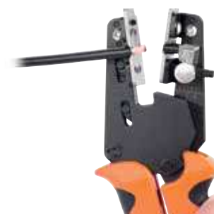
Automatic removal of insulation
