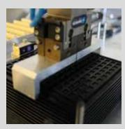
Optical presence detection of electronic trays
