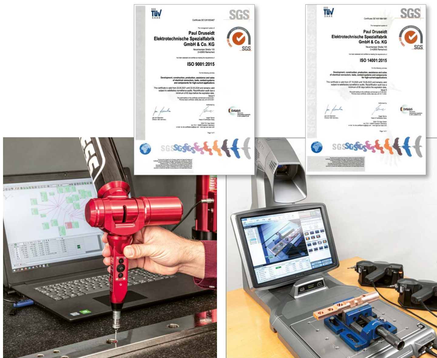
Checking the dimensions by means of a 3D-measuring arm
