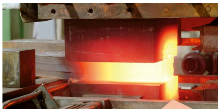
Pressure welding process for copper connectors
