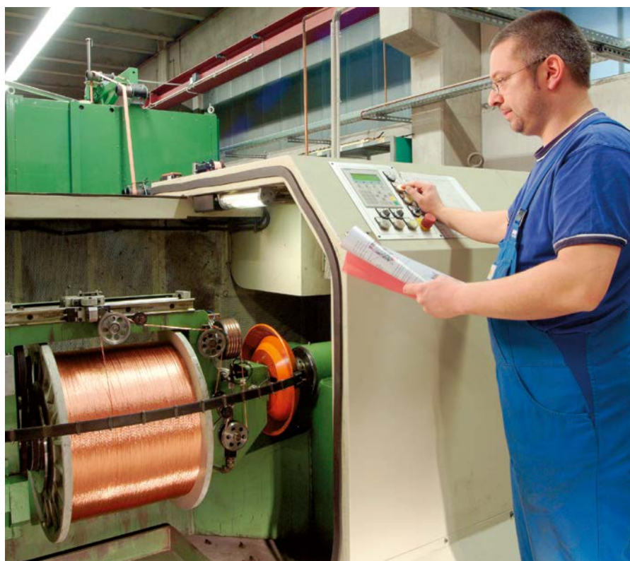
Twisting and stranding of highly flexible conductors
