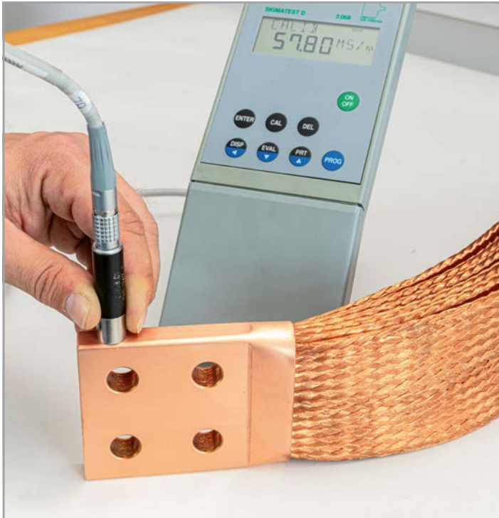
Conductivity test/flexible braided connectors
