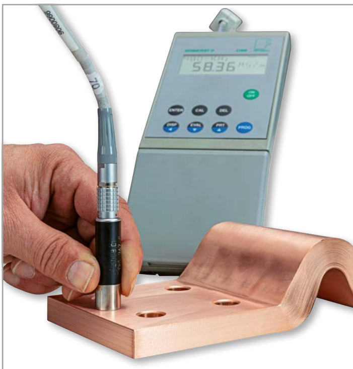
Conductivity test/flexible foil-connectors
