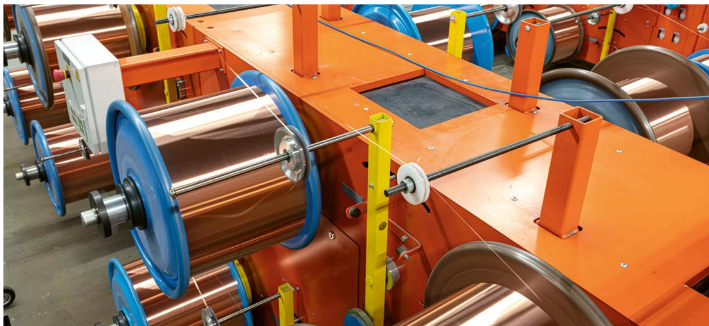
Manufacturing of round- and plait braided cables
