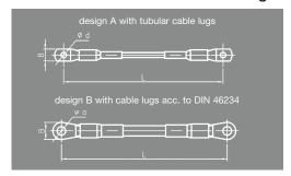
Highly flexible connectors manufactured by single insulated extruded silicone cables acc. to page 2 of these product information. Design A with tubular cable lugs. Design B with cable lugs acc. to DIN 46234. The values about the current load are in accordance with VDE 0298 Part 4 table 15.
