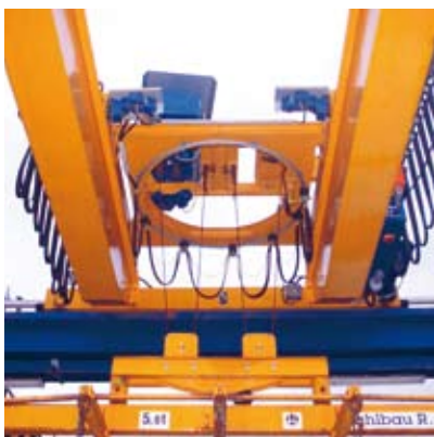
Supply of the turning-cab on an EOT-crane
