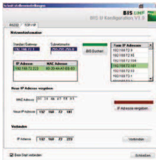
The BIS U-6027 processor and the controlling system communicate via Ethernet. Assigning a unique IP address associates the processor with a network.
