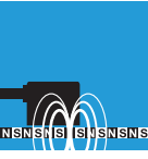
Magnetically coded position and angle measurement system
