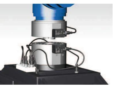
For robotics, the inductive IO-Link coupler in the compact 40×40 housing is ideal. It combines rapid format changes, freedom of wear and great flexibility. Inductive couplers eliminate the need for mechanical plug contacts, since they contactlessly transmit signals – absolutely reliably.
