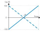
Output signal can be inverted via programming inputs.
