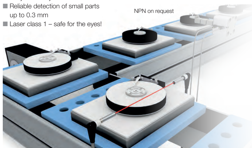
Position monitoring in an assembly line for hard drives
